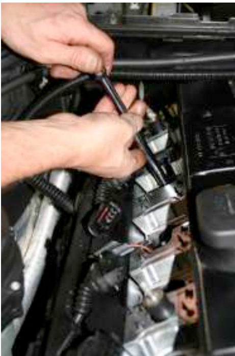
Replacing spark plugs in an M54 engine.
