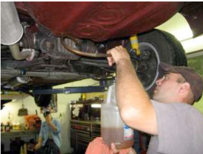
Mike Holmes fills the author's 320i differential with Red Line 75W-90 at the Former Helmut's German Auto Service in Windsor, Vt.
