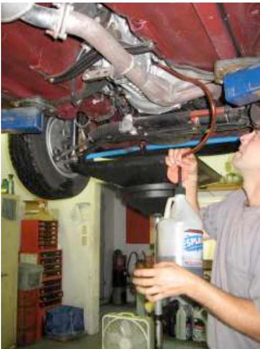
Mike Holmes fills the author's 320i five-speed gearbox with Red Line MTL at the former Helmut's German Auto Service in Windsor, Vt.
