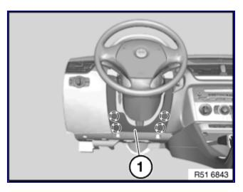
Remove clamps (highlighted area) from steering column shroud (1).
