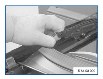
Carefully unclip left and right water channel bracket from the mechanism.
