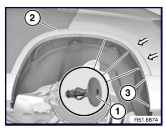
Partially release cover on wheel arch (2) left and right:
