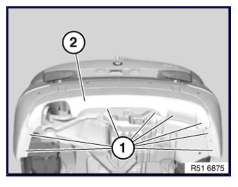
Undo screws (1) on bumper panel (2).
