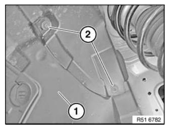
Release screws (2) on wheel arch cover front (1).
