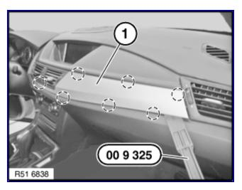
Lever out the cover (1) on the marked points with special tool 00 9 325.
